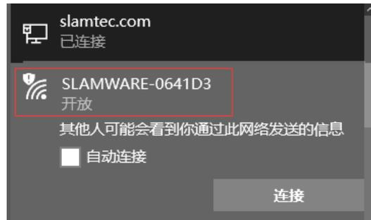
Please connect to the above SLAMWARE- XXXXXX with the wireless card (you can also connect Breakout to PC with wired network, in this condition, please set the network mode as DHCP). Then open the application uicommander.exe in the bin folder of SDK packet, the default ip address is 192.168.11.1. If connecting success, there will be the scanned map by RPLIDAR in the uicommander.
